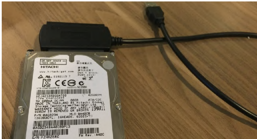
109. Hard drive from the PCS Programmer connected to USB/IDE adapter
