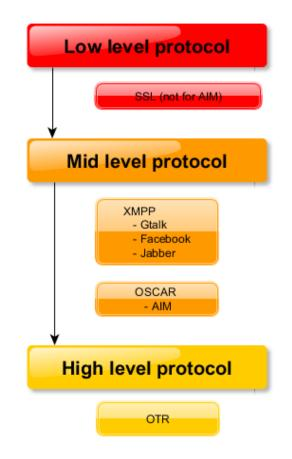
Basic XMPP protocol is not protected against MitM and replay attacks. SSL usage offers a good protection but not end-to-end and Google / Jabber / Facebook servers could intercept all traffic in cleartext before sending back the XMPP packet over SSL to the remote user. That's why OTR protocol has been chosen, mainly to ensure even instant messaging servers could not spy users' messages.
